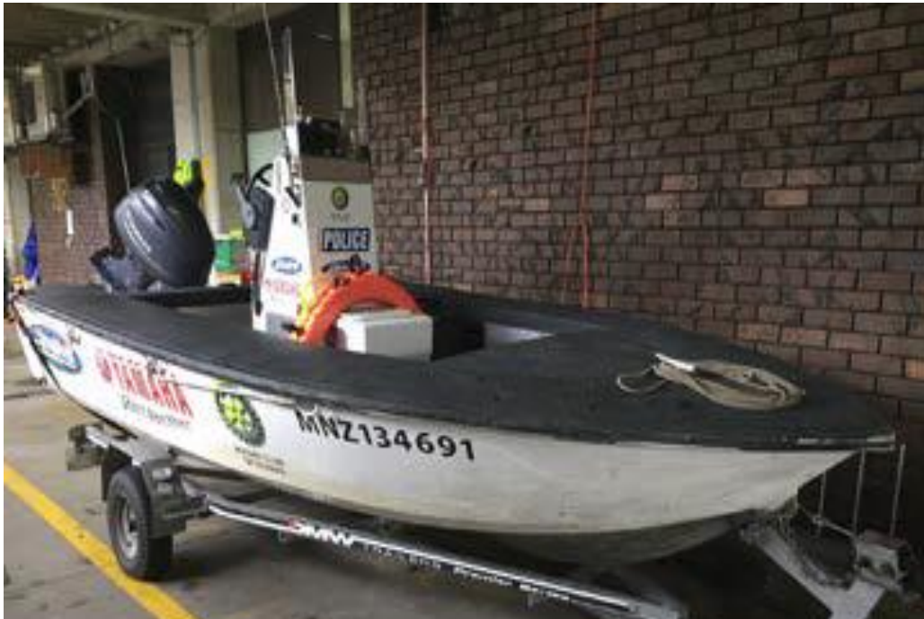
The Hamilton Police boat. The central console contains the boat controls and the Police radio.
